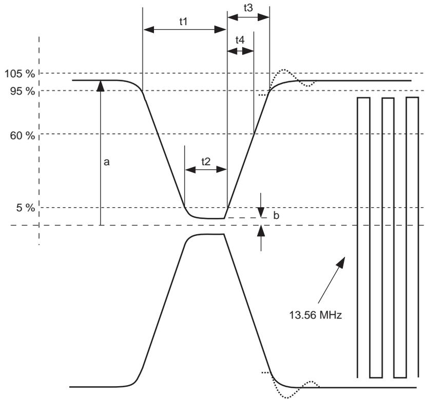
Maximum and minimum values of  $t_1$ ,  $t_2$  and  $t_3$  are specified in "■ RECOMMENDED OPERATION CONDITIONS".  $y$  is 0.05 ( $a-b$ ) and the maximum value of  $hf$  and  $hr$  is  $0.1(a-b)$ .
