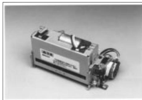
**FTP-631MCL301/302 shown after assembly with FTP-631CT001cutter**
